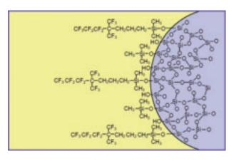
Figure 1. Schematic surface model of Fluofix
